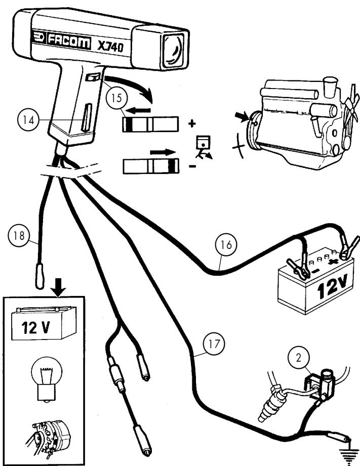
Start the engine and check that it is running at its idle speed. Turn on the stroboscopic function lamp ⑩ by pressing the key ⑤. Direct the flashing lamp onto the flywheel window by pressing the trigger ⑭. Turn the knob ⑯ to make the flywheel mark line up with the 0° mark on the housing. Release the trigger ⑭ to hold the figure in the display ⑧ for 10 seconds. Read the initial timing figure on the display ⑧ and compare it with the manufacturer's figure.
